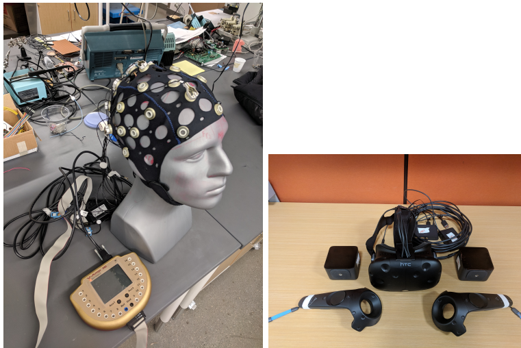
Figure 1: Pictured are the Brain Products V-Amp/ActiCap Xpress system (left) and HTC virtual reality headset/controllers (right)
